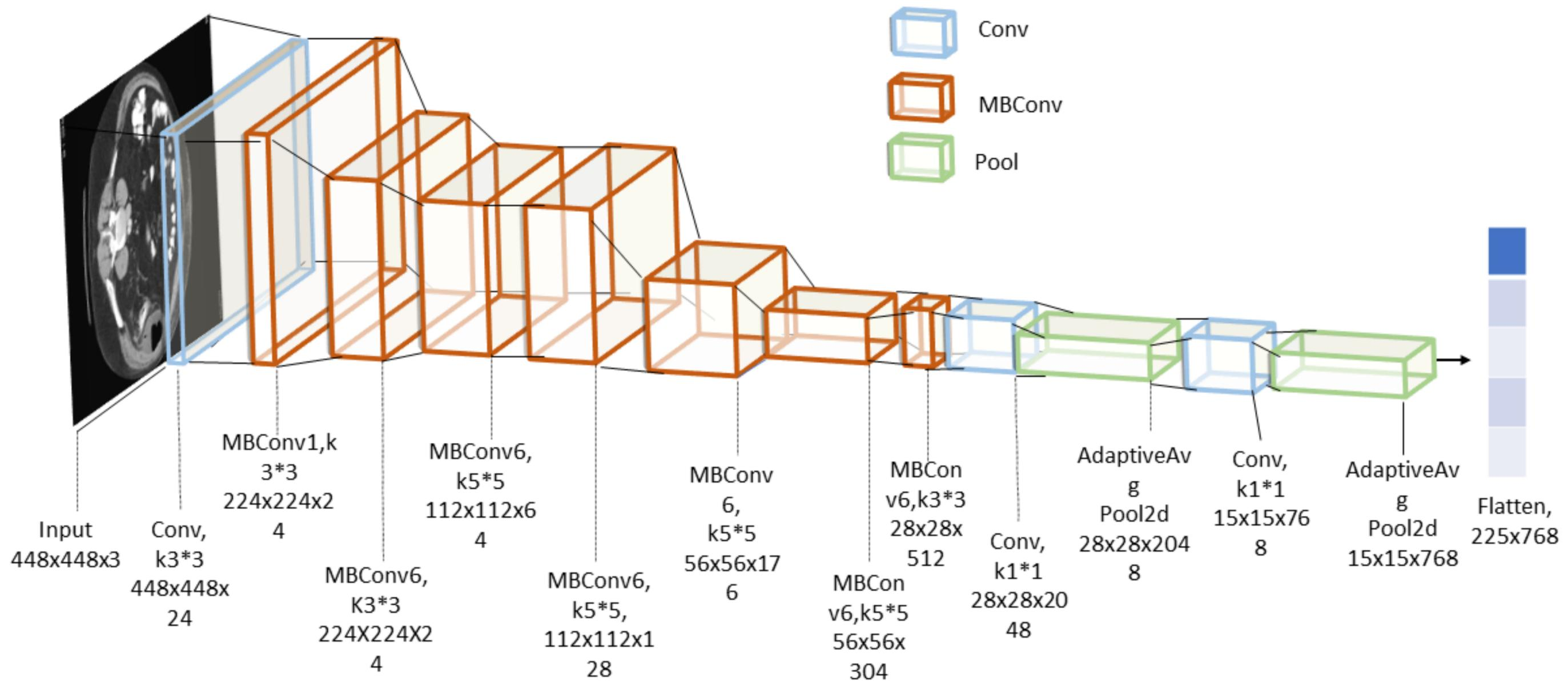
The architecture of EfficientNet-b5 model
