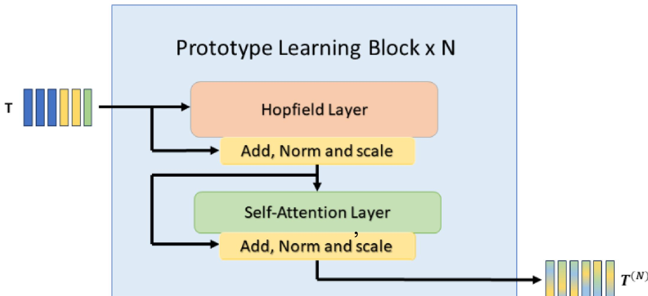
Figure: Detail of Prototype Learning Block.
