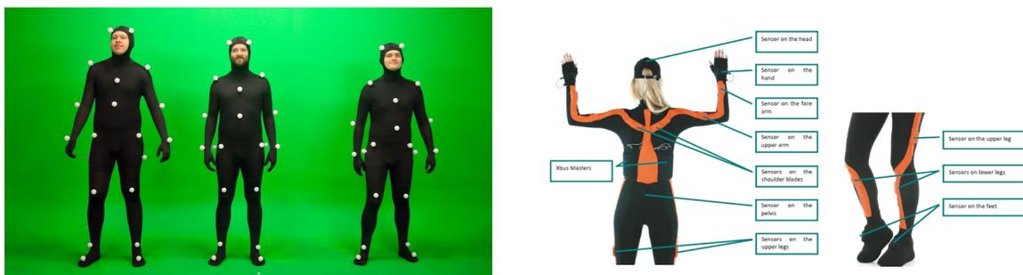
Fig. 1.1 Setup for Computer Vision (left) and setup with IMU sensors (right).
