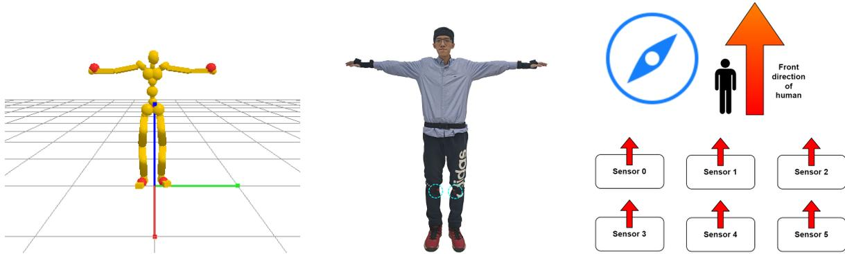
Fig. 4.10 Setup of T-pose in GCS and VCS. At left is the character at T-pose in simulation, center is human at T-pose and right is set 6 IMU sensors when defining front direction.
