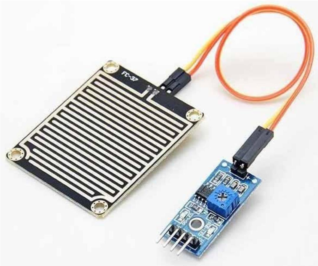
**Figure 3.8: Rain drop sensor**
