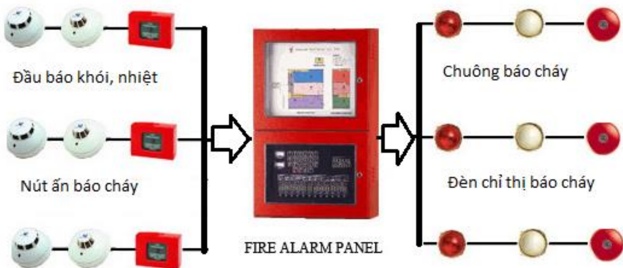
Basic Fire Alert system components
