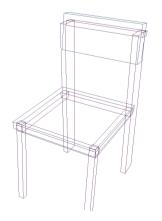
**Figure 3-10** A chair modeled in 3-D is made up of various blocks and rectangles.
