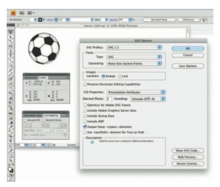
**Figure 3-8** Drawing software such as Adobe Illustrator can save vector graphics in SVG format.
