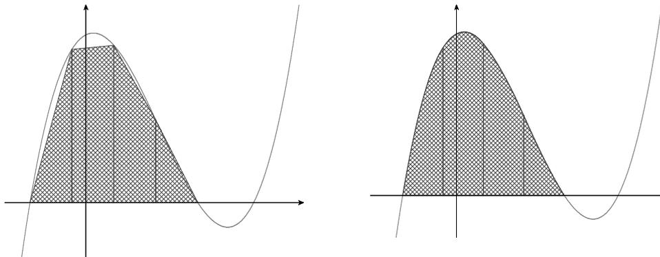
Figure 2. Trapezoidal formulas (left) and Simpson methods (right)
