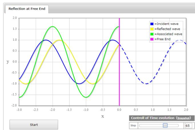
Figure 2. The simulator of free end reflection of a sine wave.
