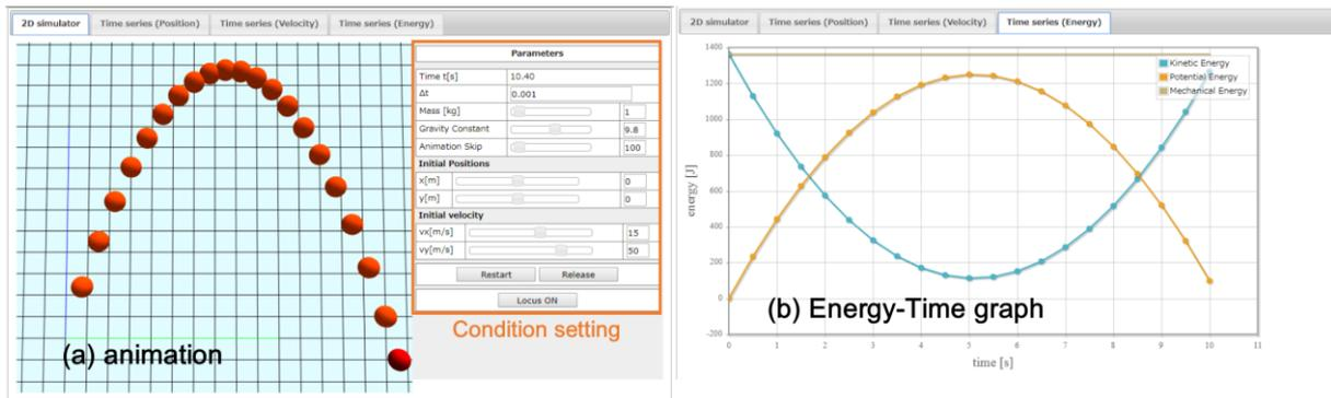
Figure 2. The simulator of the falling motion with animation (a) and Energy-Time Graph (b).
