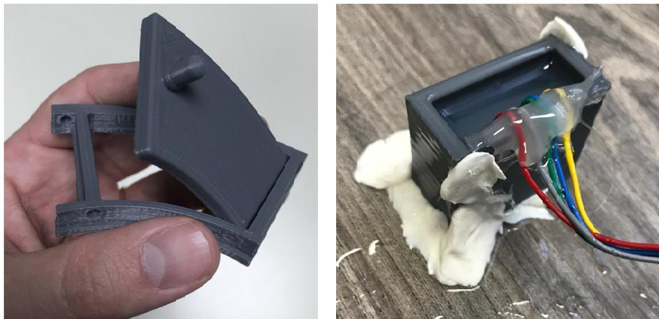
Figure 4. Some examples of the final prototypes and tests. a) Assessment of tolerances for pill dispenser. b) Sensor encapsulation in PDMS.
