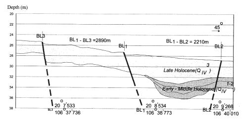
Figure 3. Echo sounder cross section in front of Balat mouth.
