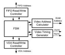
Fig. 4. Composition of the VGA Controller module.
