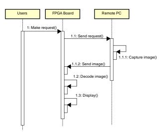
Fig. 8. Sequence diagram of the remote camera system.
