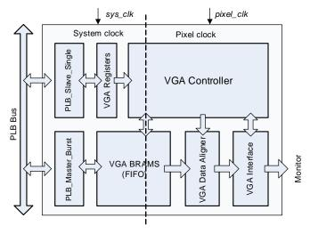
Fig. 1. VGA monitor controller architecture.
