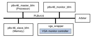
Fig. 5. Verification model for VGA monitor controller.
