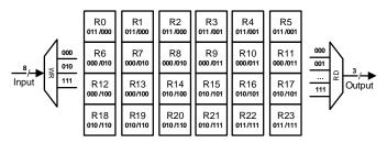
Fig. 3. VGA Data Aligner for 64 bits mode.
