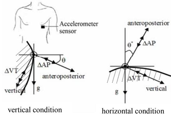
Figure 1. Sensor module location (AP: anteroposterior, VT: vertical)
