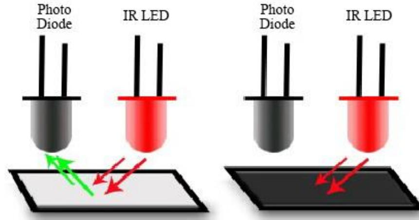
**How can the robot track a black line?**
