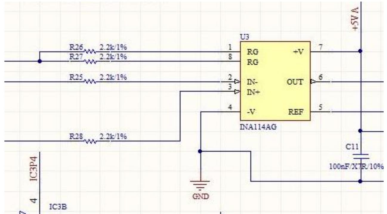
instrumentation amplifier schematic
