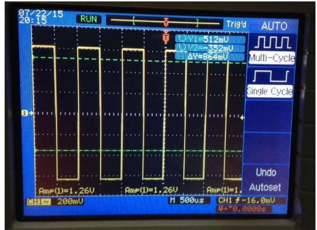
*Pulse generator, test manipulation and result displayed on oscilloscope*
