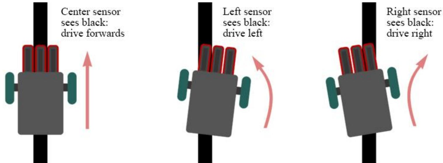
How can the robot track a black line?
